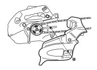
5. While holding up the tip of the bar, adjust the chain tension by turning the tensioner screw until the tie straps of chain just touch the bottom side of the bar rail
